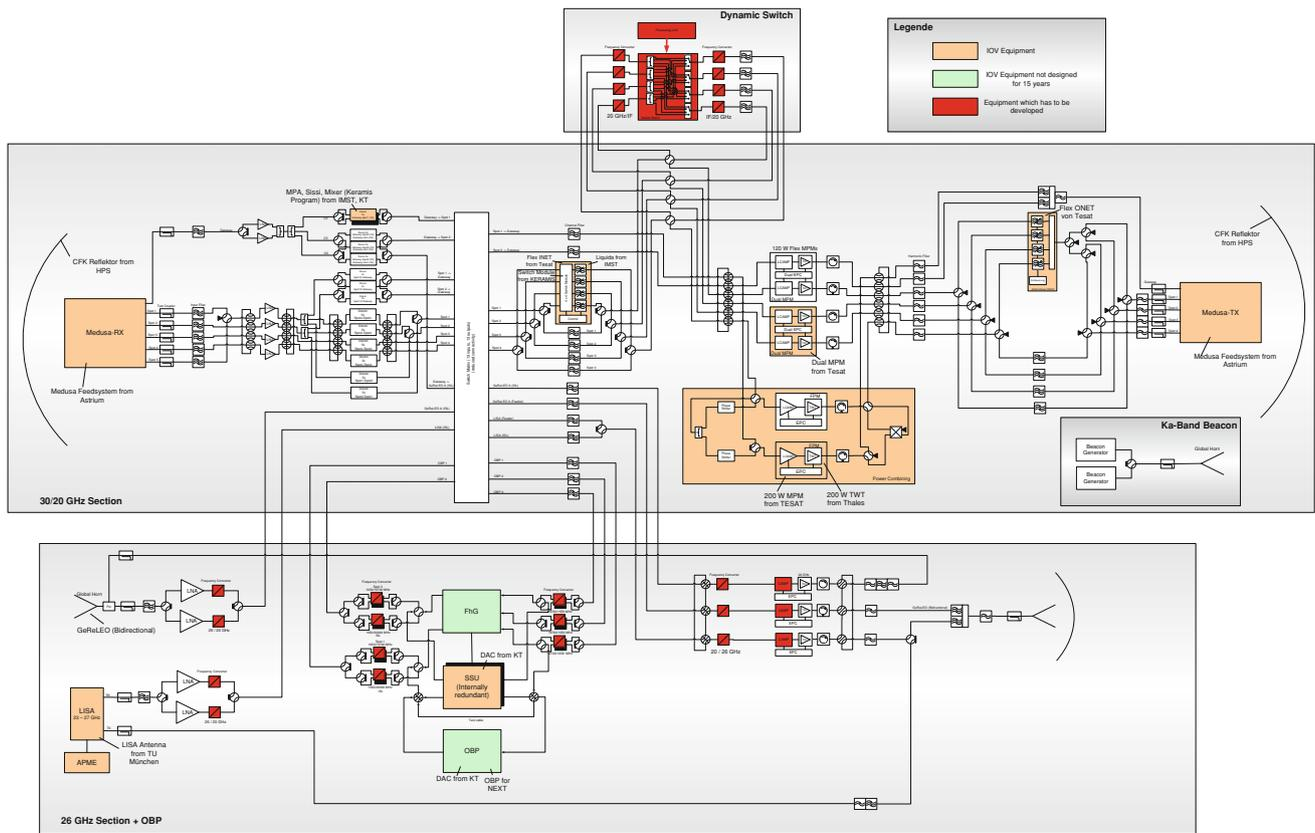
**Fig. 3** Phase A version of the communication payload for in orbit verification
