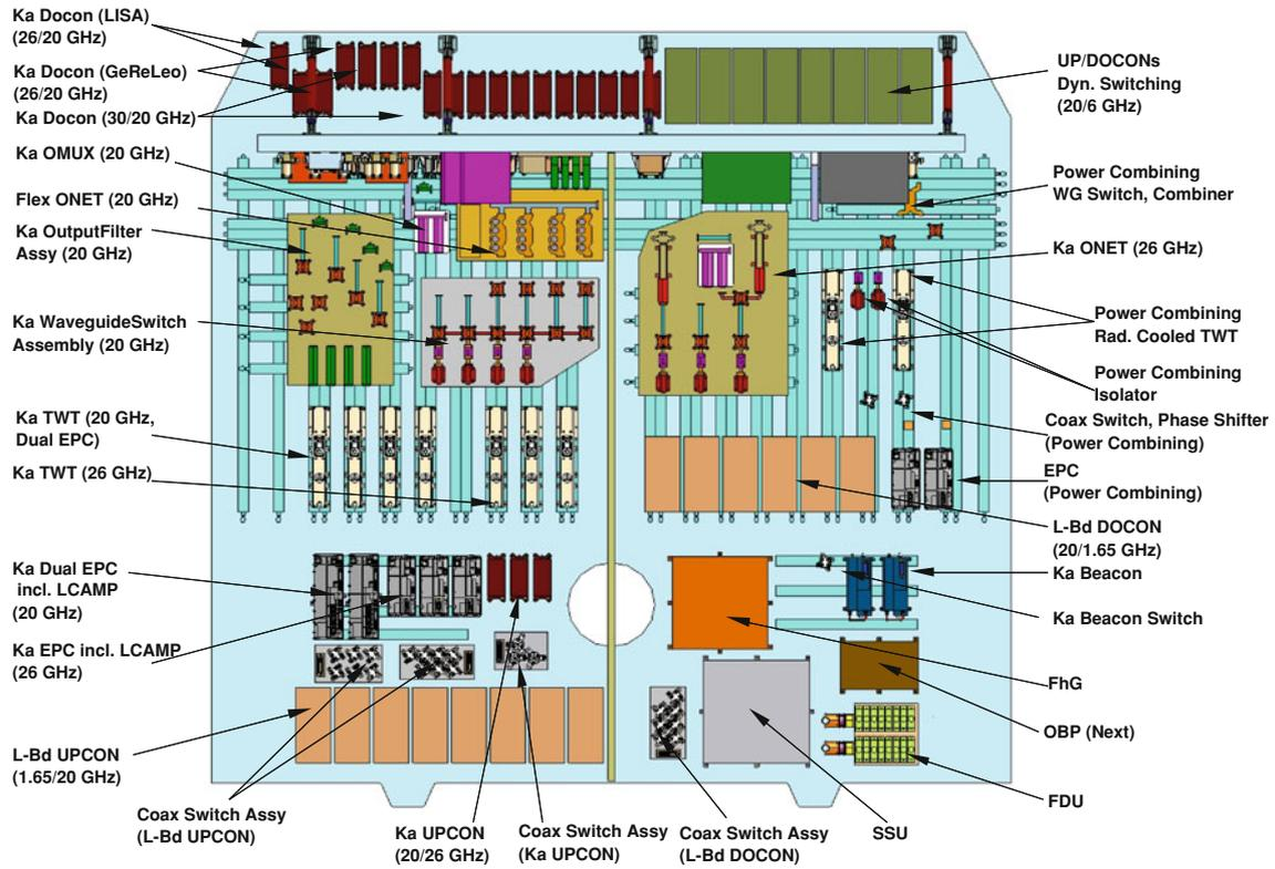
Fig. 4 Accommodation of the payload on the north panel
