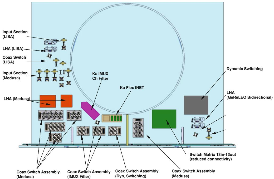
Fig. 5 Accommodation of the payload on the earth panel
